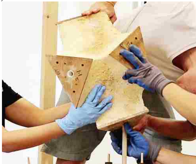
Figure 29: MycoTree component fabrication
