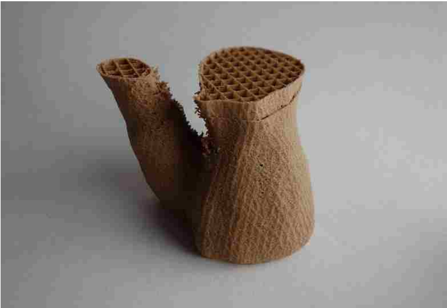
Figure 37: 3-D printed segment of straw core.
