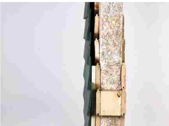
Figure 22: Mycelium insulation material
